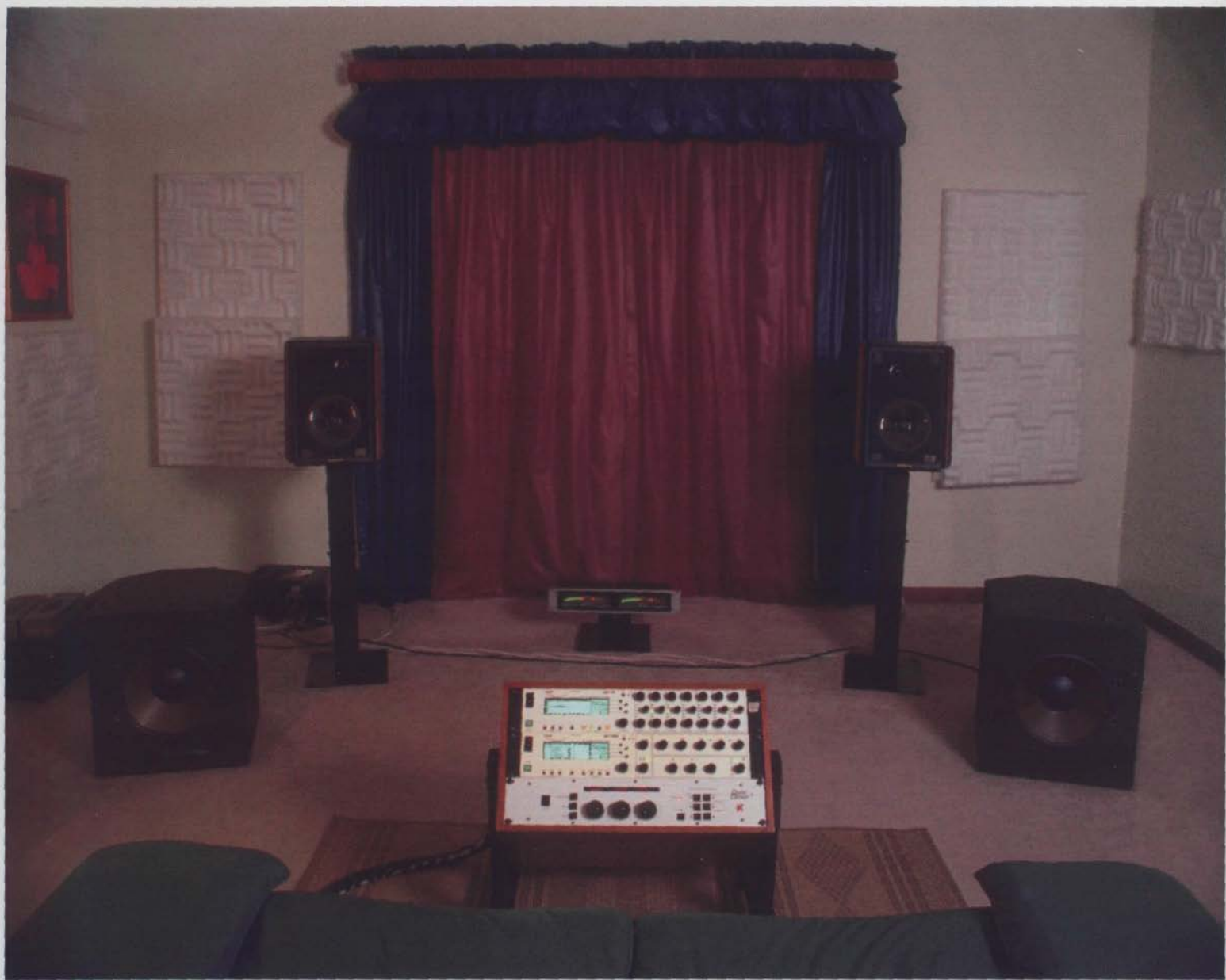
View from the bridge. Digital Domain's Mastering studio. Visible in front of the listening couch are: Rolling rack with Weiss EQ-1 LP Equalizer, Weiss DS1-MK2 dynamics processor, and Digital Domain DD-2 K-Stereo Processor; One pair of Dorrough meters; Reference 3A (satellite) loudspeakers on sand-filled stands plus Genesis Servo-controlled subwoofers.
