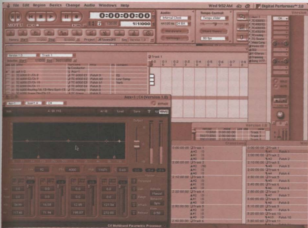
Digital Performer in action, slaved to the mastering DAW. Performer automates both external devices via MIDI and plug-ins acting as outboard processors to the main workstation, for example, SADiE.
