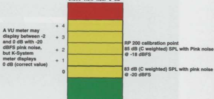
Figure C15-02: A K-20/RMS meter in close detail, with the calibration points.
