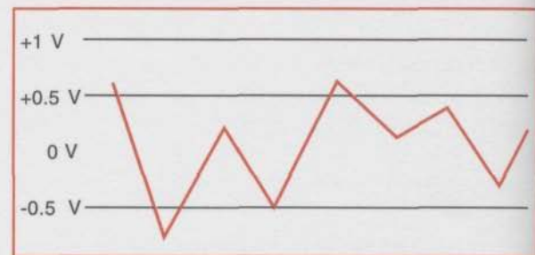
Random dither applied to the ADC whose highest peak-to-peak value is slightly greater than the LSB and whose average value is zero volts.
