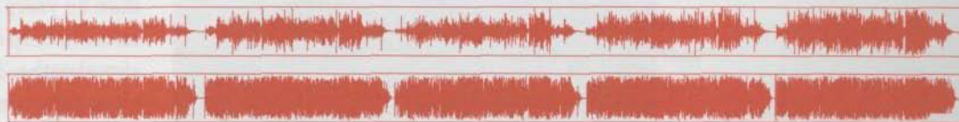
At top, five mastered cuts of the same music, with increasing loudness and visual density. At bottom, the same cuts passed through the Orban radio processor. 1
