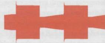
Output of a Compressor with a low ratio, slow attack time, slow release time plus release delay
